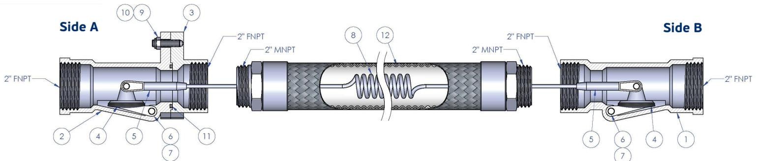
1. Step 1 – Thread LifeGuard Fitting A onto **Side A** of hose and insert patented Safety Spring through bore of hose;
